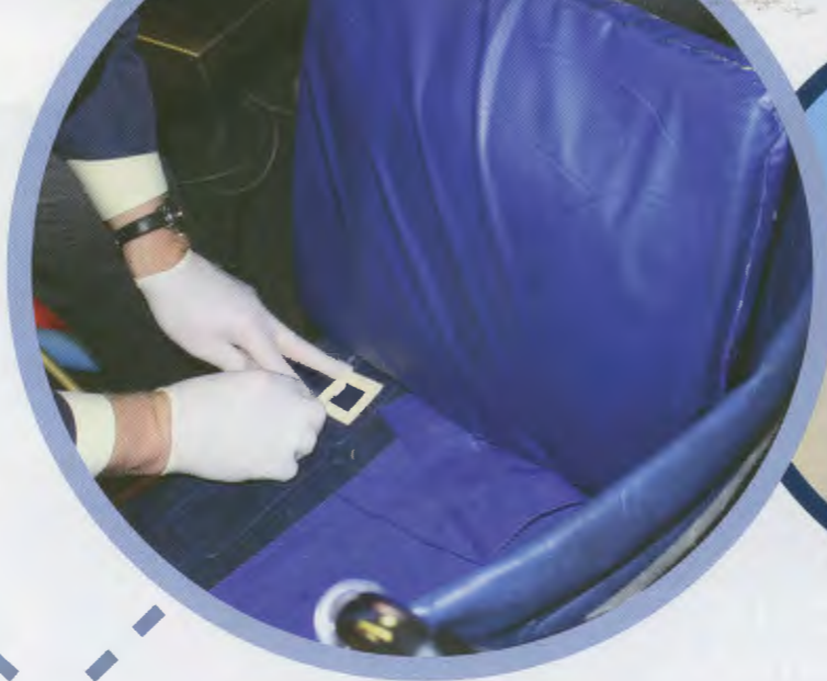
Both the seat and the seat cushion of a wheelchair were tested. Testing showed a substantial reduction of bacterial contamination from the various surfaces.
