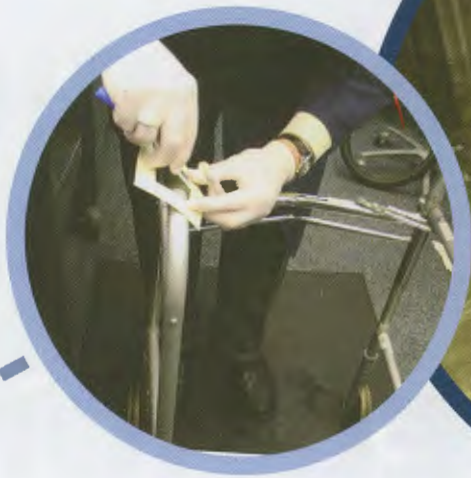
Flexible templates allowed sampling of irregular surfaces. This photo shows a post-cleaning sample being collected from a walker.
