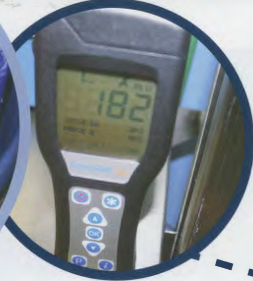
The pre-cleaning result for the wheelchair cushion was recorded on the BioReveal unit at 182 relative light units (RLUs).
